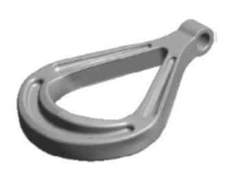
The Permanent Chain Chaser is used on semi-submerged rigs to prevent anchors from having to be buoyed off for recovery. The material of the Permanent Chaser is softer than the wire or chain. This is to make the chaser sacrificial between the two so that the chain or wire does not get damaged. This is used as an alternative to the buoy and pennant.
